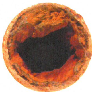
Figure 2-1 Galvanized Steel Distribution Main Removed from the Port St. Joe Distribution System in early 2010
